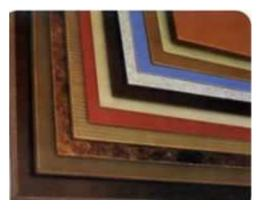
Technical laminates are produced in the form of plates, tubes and sticks as follows: Based on phenol resin; Paper - PEPERPHENOL; cotton - TEXTILEPHENOL; On the basis of epoxy resin and glass fibers - EPOXYGLASS: Mica based flexible and rigid materials-
